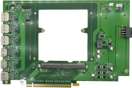
The **SX-MXM-TOOL** is an PCIe adapter supporting MXM 3.1 Type A, Type B, and Type B+ GPU modules for quick validation and early development purposes on your AI applications. The modules are supported All MXM GPUs solution
